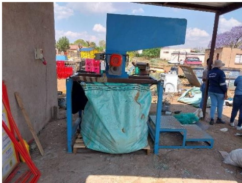
Figure 4-24: Glass crusher facility
