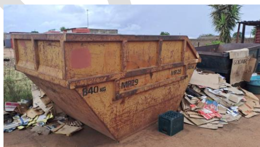
Figure 4-31: 9m 3 skip used for recyclable materials
